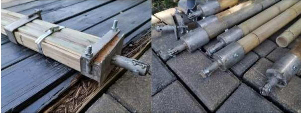
Fig. 6. Nozzles for bamboo splits and culms after being installed, and ready to be fabricated. There are also the design of straps for bamboo split bundles, similar to nozzle for splits.
