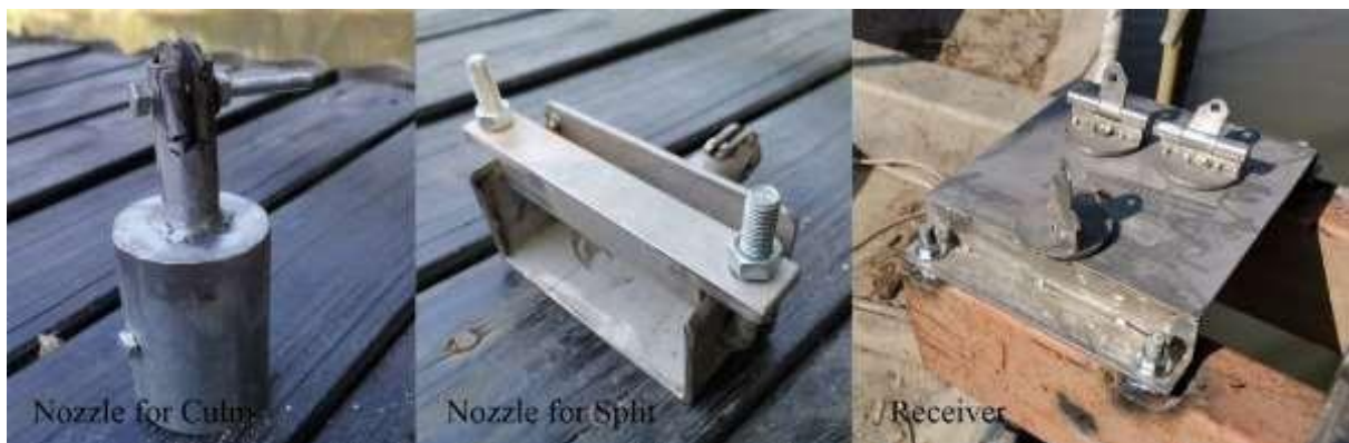
Fig. 5. Images show different designs of nozzles and receiver for bamboo structural joints
