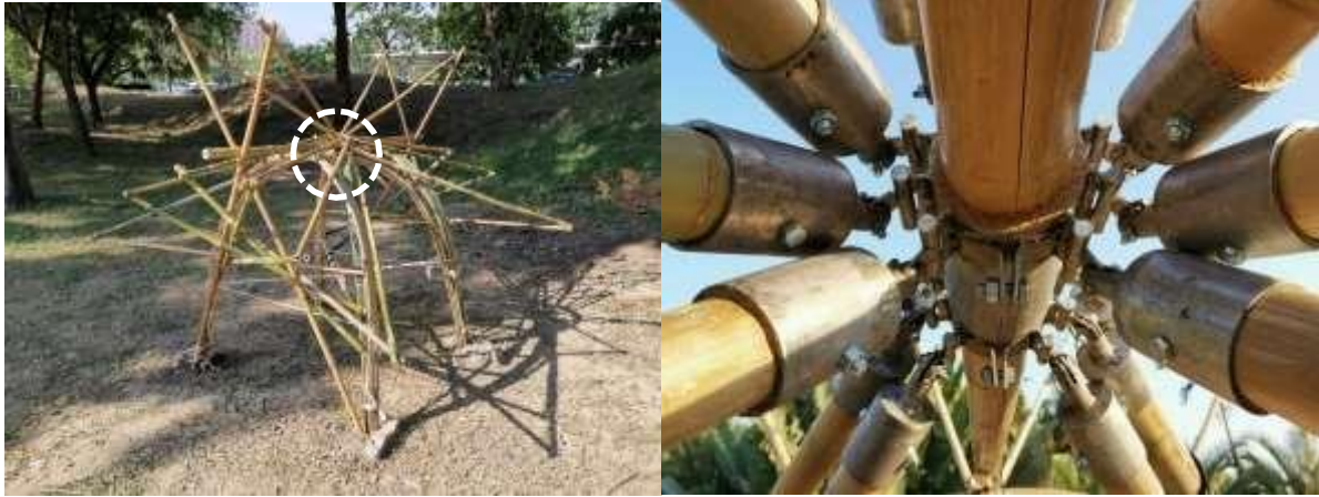
Fig. 4. (Left) The model of prototype design was created to study the potential way to design connectors. (Right) Model helps the understanding of the connector at the hub.
