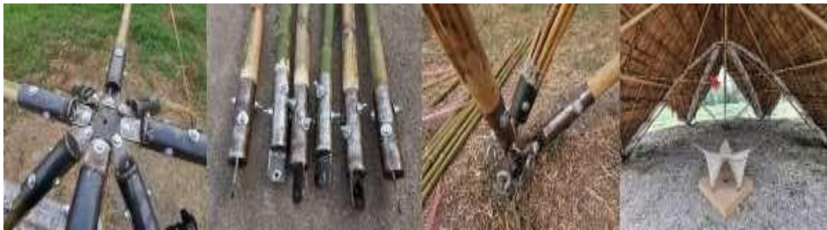
Fig. 16. Carrying on Experiment to re-design nozzles and star plates and build a simple structure by Thammasat Bamboo studio.
