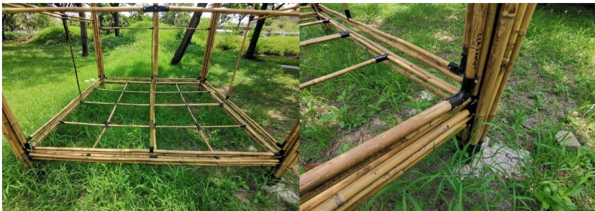
Figure 22. Experiment of using commercial connectors in industry by applying the use with bamboo to construct the prototype shelter.
