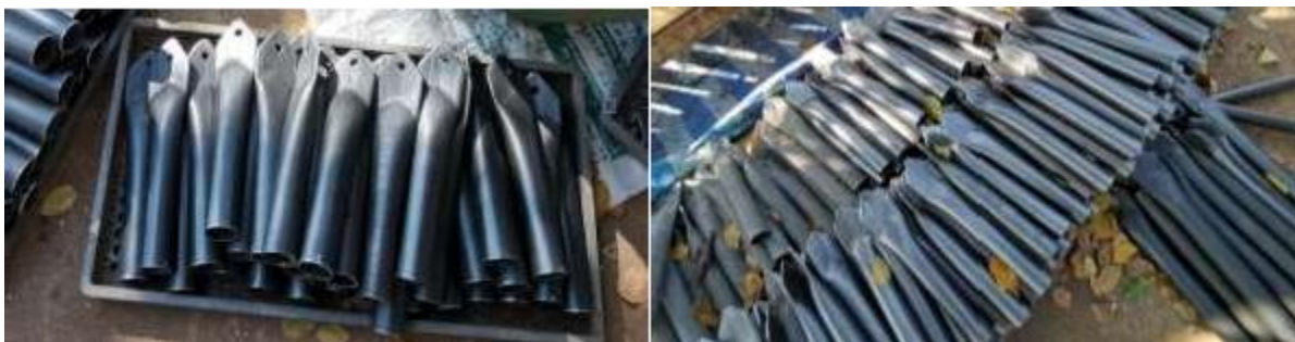
Fig. 12. Head nozzles are produced mass production, since the truss frame will be made of
