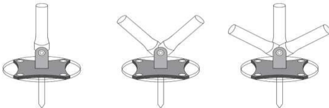
Fig. 11. The star plate at node connecting to the ground or foundation.
